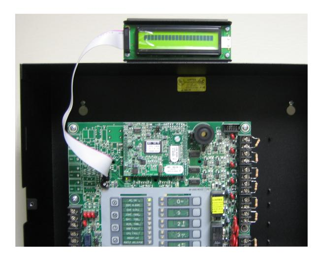
CFG-300 attached to main board
